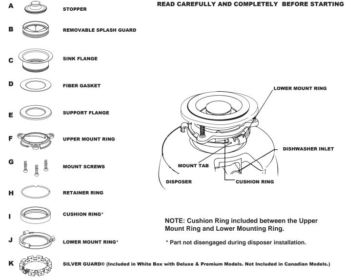
NOTE: As the mounting assembly is properly assembled at the factory, please pay close attention to the order of the mounting system parts.
